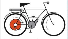
**Rear hub motor** Rear hub motors provide power to the bike's back wheel, 'pushing' the cyclist along the road
