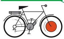
**Front hub motor** A front hub motor spins the bike's front wheel, making it feel as though the bike is being pulled
