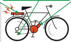
**Mid-drive motor** For a more conventional ride, mid-drive motors sit on the frame and send power to the drivetrain
