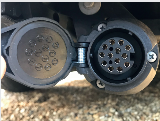
Inspect the 13-pin socket and coat it with a water-inhibiting product
