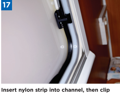
Insert nylon strip into channel, then clip in drive block and side catches. Finally, replace stay-bracket and end-stop screw
