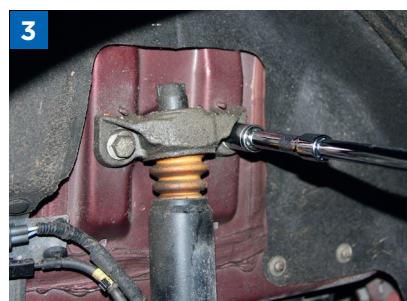
3 Removing the upper shock absorber mounting bolts
