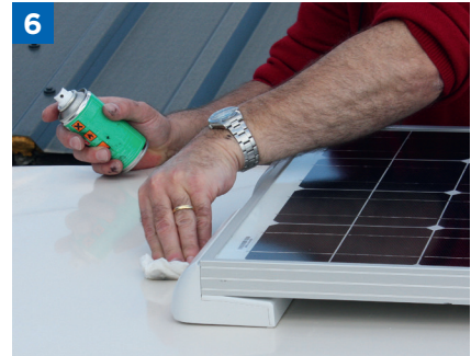
6 Clean off any excess adhesive
