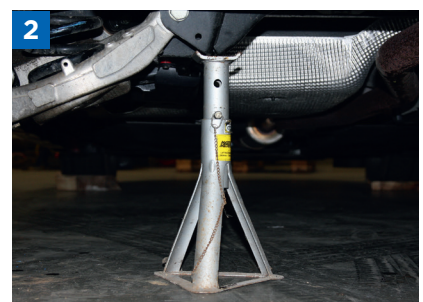
2 The rear of the vehicle supported on axle stands for the procedure
