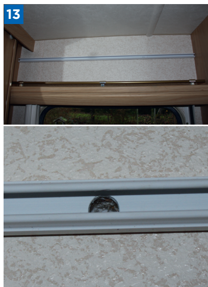
13 New trunking inside the caravan behind the light unit; 8mm hole in the trunking
