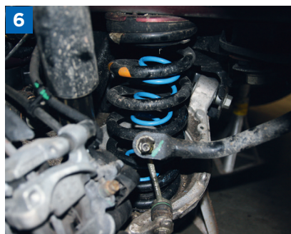
Auxiliary spring inserted into main spring
