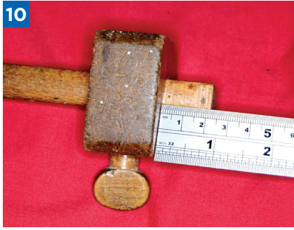
Set marking gauge to the required width (17mm in this example)
