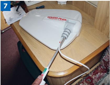
Wind the 'gearbox' to 90 degrees
