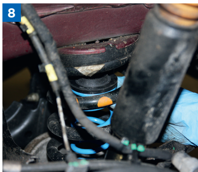
The upper spring seat in position
