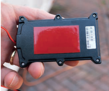
Reverse side of the DB2 device, showing the pre-attached double-sided tape
