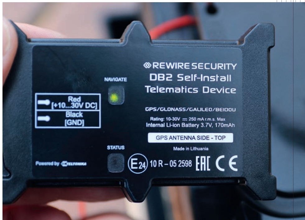
Solid 'Navigate' light, searching for GPS, with flashing 'Status' LED
