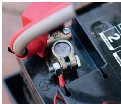
Red (positive) wire from DB2 connected
