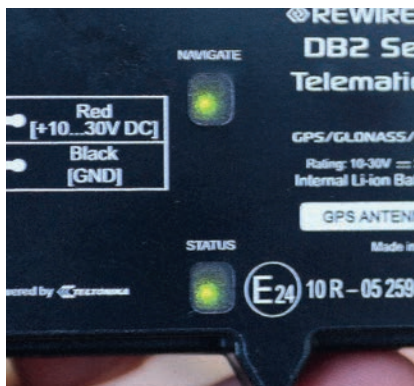
Both LEDs flash, showing DB2 is operational
