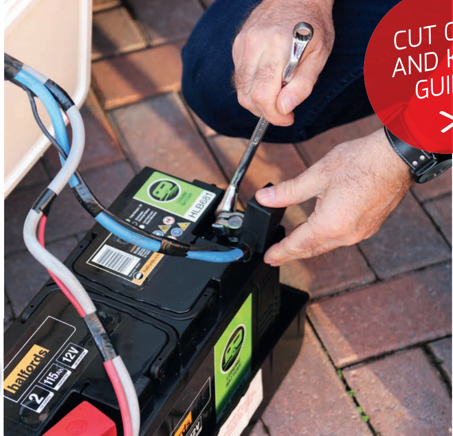
Loosening the battery terminal nut
